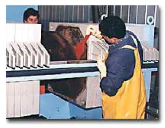
At Patagonia Salmon Farms in Puerto Montt, Chile, workers remove the dry filter cake from a Beckart Environmental Hy-Pack Filter Press at the end stage of the wastewater treatment process.
